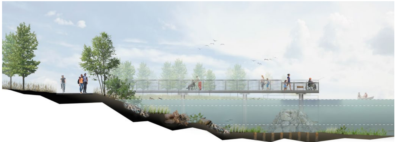
The K&T Trail Living Shoreline project proposes removal of 500 feet of concrete bulkhead and replacement with a dynamic, gently-graded riparian landscape near the Tacony Boat Launch.
