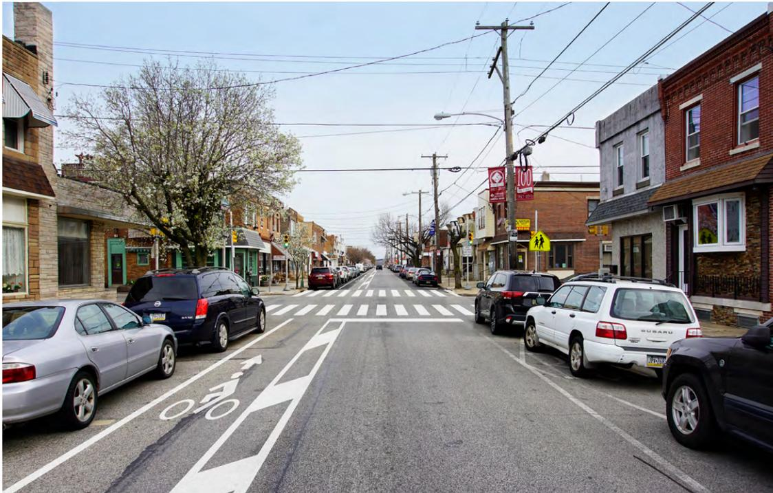
*A rendering of a potential buffered bike lane on Orthodox Street.*
